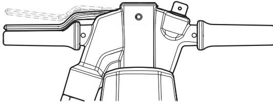
Continue to press the start and stop device all the way down to activate full power of the pneumatic breaker.
