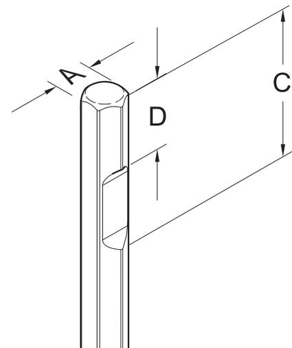
Use the gauge that corresponds to the insertion tool's shank dimension. See section "Technical data" for correct tool shank dimensions.
